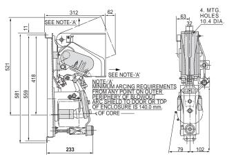
MINIMUM ARCING REQUIREMENTS FROM ANY POINT ON OUTER PERIPHERY OF BLOWOUT ARC SHIELD TO DOOR OR TOP OF ENCLOSURE IS 139.7 mm
