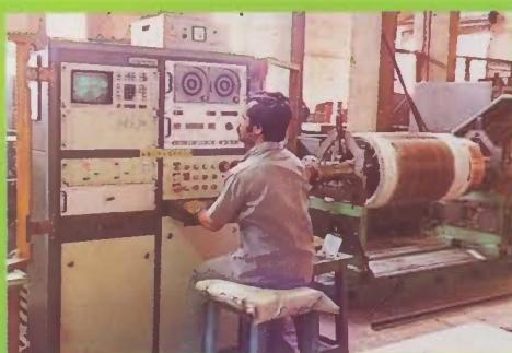
Armatures are dynamically balanced to precision grade to ensure low vibration operation.
