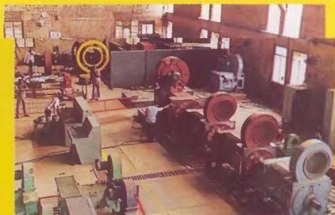
Thyristor converter source of supply is employed for testing all motors to ensure the satisfactory performance of the machine on both thermal levels and commutation; under influence of ripple content. Simulation of application conditions for acceleration, braking, reversals and starting can be demonstrated.
