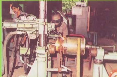
Choice of TIG-Welding joints for the armature coil to Commutator is available when very high currents are involved.
